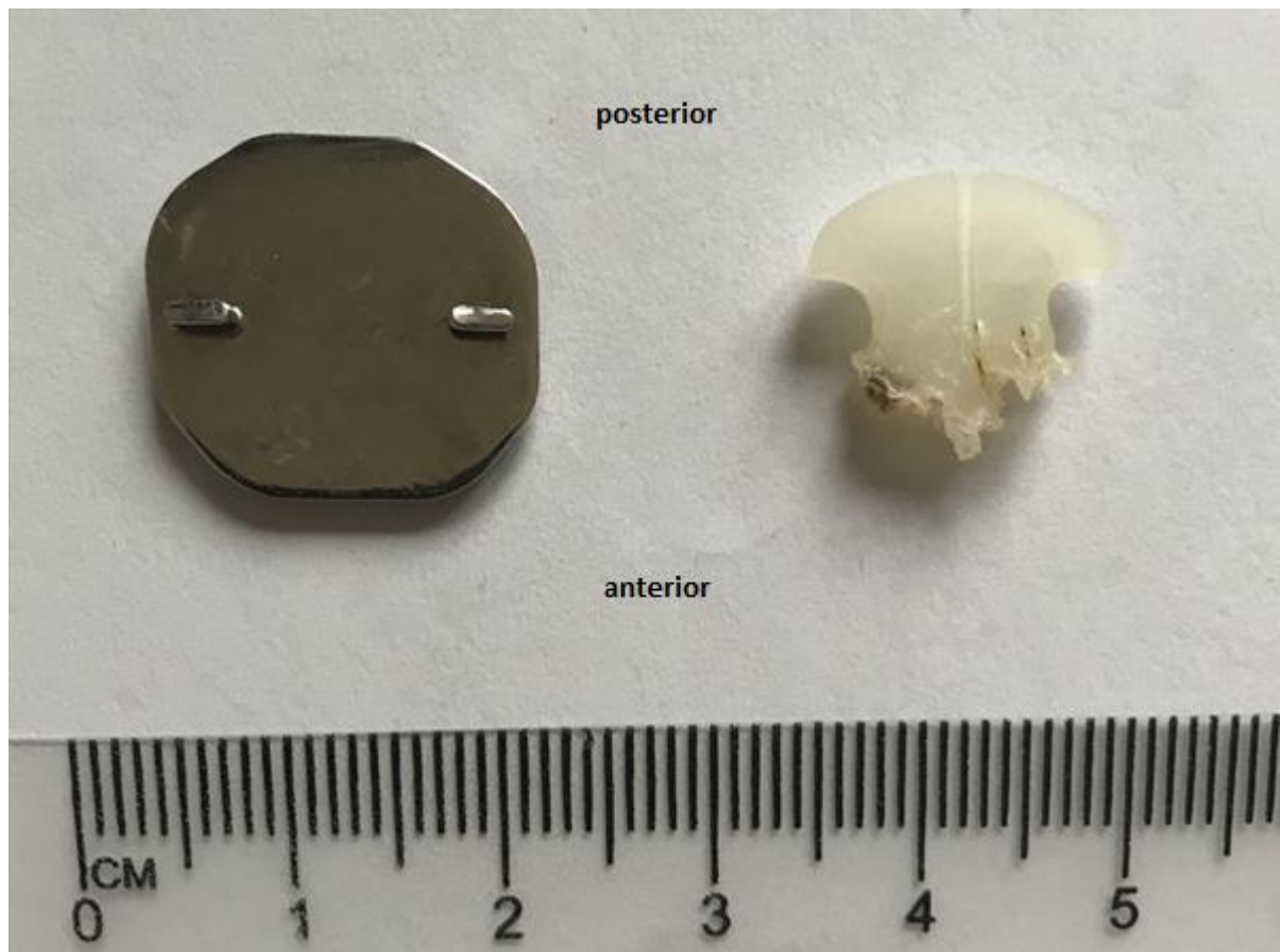
Figure 10 The inferior CoCr plate and the flat surface of the UHMWPE insert, respectively.
