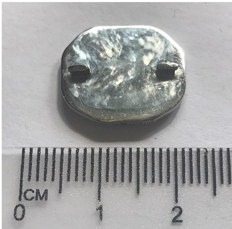
Figure 12 The articulating surface of the inferior CoCr endplate.
