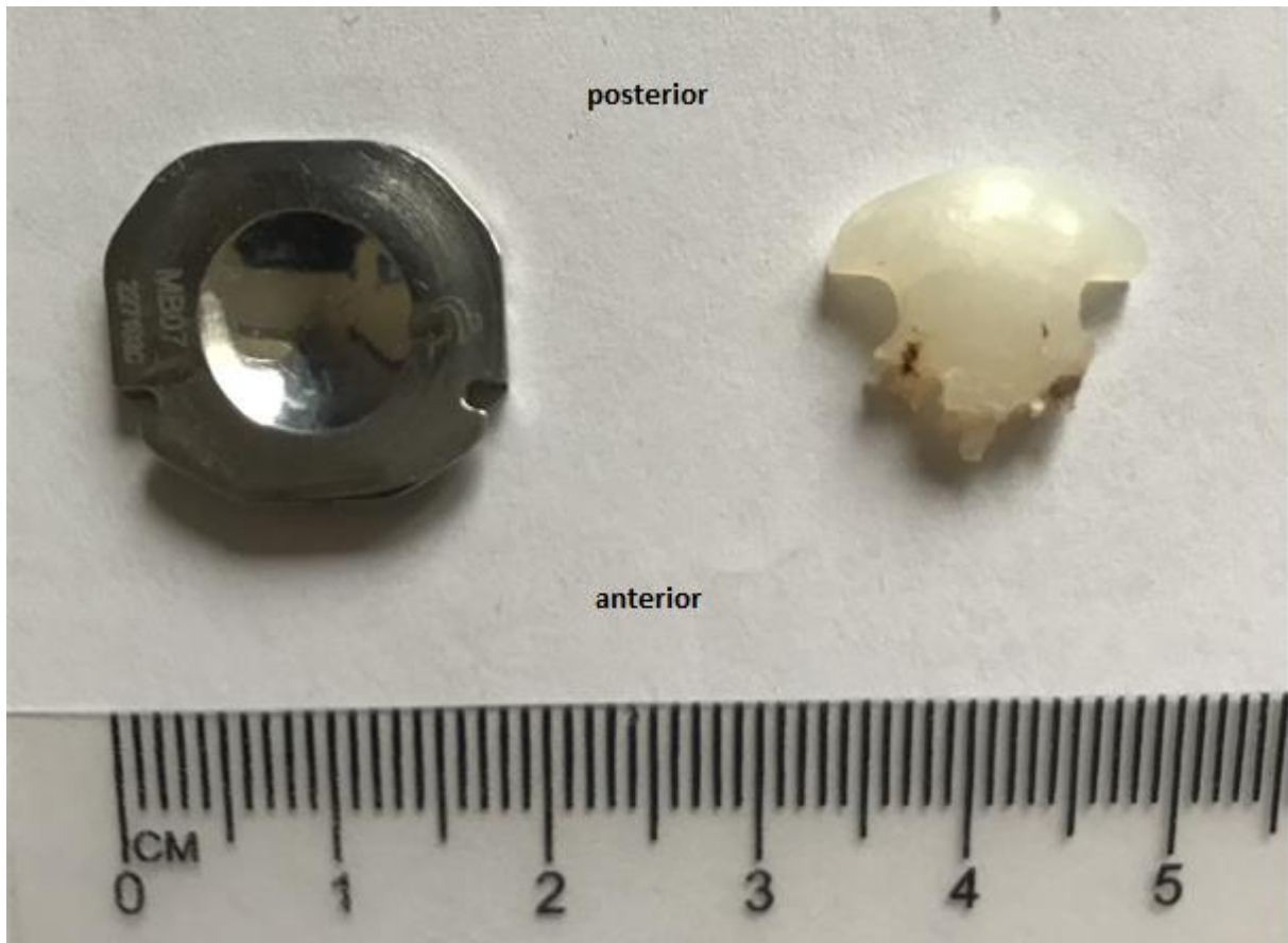
Figure 13 The superior CoCr plate and the curved surface of the UHMWPE insert, respectively.
