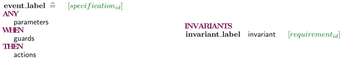
Fig. 2. An example of annotated Event-B model event and invariant in the Rodin platform
