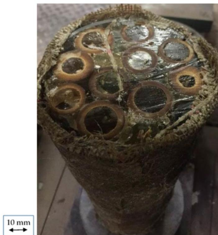
**Figure 1.** Physical composite constructed of full culm Moso bamboo fibres, epoxy matrix, and PVC confinement that the model in the present paper is based on Mofidi et al. [3].
