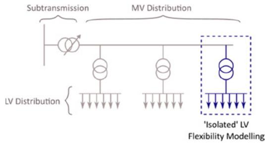
**Fig. 1** Isolated LV flexibility modelling does not consider the coupling of voltages that occurs on MV distribution lines (although a Thévenin impedance models the impedance of the MV distribution circuit to an individual feeder)
