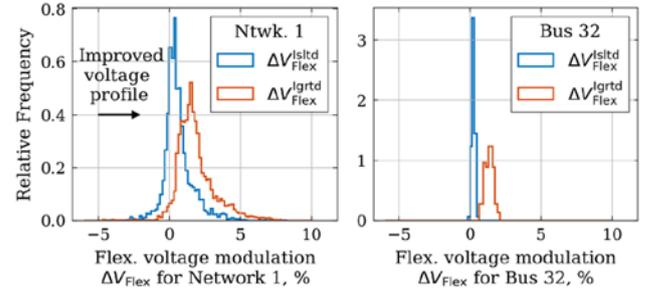
**Fig. 7** Histograms of the flexibility voltage modulation for Network 1 (left) and Bus 32 (right) between the hours of 16:00 and 21:00, comparing the isolated flexibility voltage modulation  $\Delta V_{Flex}^{Isld}$  against the integrated flexibility voltage modulation  $\Delta V_{Flex}^{Igrtd}$
