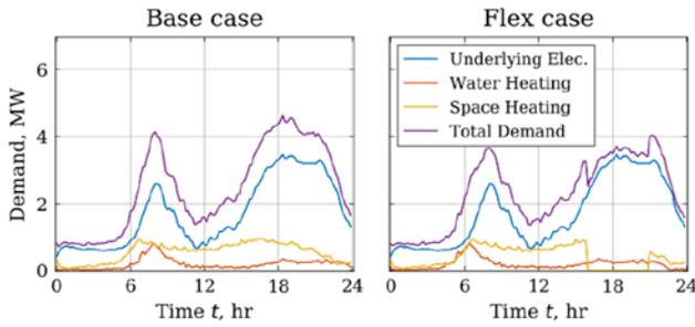
**Fig. 4** By shifting the water heating demand schedule forward by 90 min and using gas for space heating from 16:00 to 21:00 h, the peak demand from the base case (left) is reduced in the flex case in both the morning and the evening (right)
