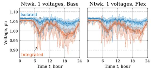
**Fig. 6** Comparing the isolated and integrated models in terms of the range, IQR and median LVs; these are plotted for the base case (left) and flex case (right)
