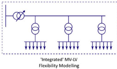
**Fig. 2** Integrated MV-LV flexibility modelling explicitly models all coupled circuits, to calculate the full realisable benefits of flexibility actions on voltage magnitudes
