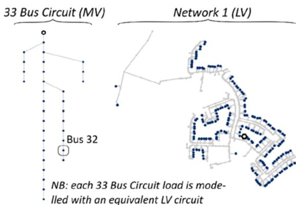
**Fig. 3** 33-Bus circuit of [6] (left) is coupled with 32 LV networks from [7], with Network 1 (right) connected to Bus 32
