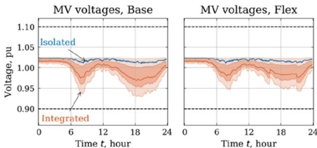
**Fig. 5** Comparing the isolated and integrated models in terms of the range, IQR and median MVs; these are plotted for the base case (left) and flex case (right)
