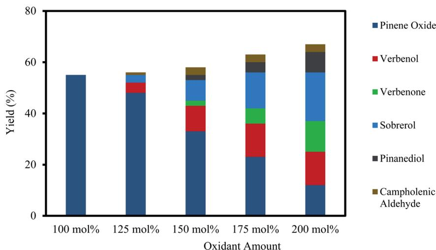
Fig. 4 Effect of the oxidant amount on  $\alpha$ -pinene epoxidation and the distribution of the products. Reaction conditions: temperature ( $50^\circ\text{C}$ ), reaction time (120 min),  $\alpha$ -pinene (1.25 M),  $\text{Na}_2\text{WO}_4 \cdot 2\text{H}_2\text{O}$  (0.012 M),  $\text{H}_2\text{SO}_4$  (0.05 M) and toluene (500 mol%).
