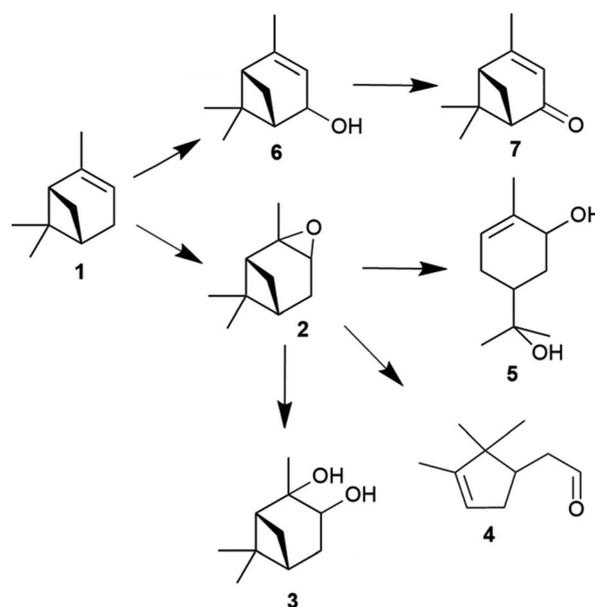
Fig. 1 Products obtained from the epoxidation of  $\alpha$ -pinene with hydrogen peroxide ( $\text{H}_2\text{O}_2$ ) catalysed by tungsten-based polyoxometalates;  $\alpha$ -pinene 1,  $\alpha$ -pinene oxide 2, pinanediol 3, campholenic aldehyde 4, sobrerol 5, verbenol 6 and verbenone 7.
