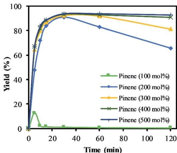
Fig. 7 The yield of  $\alpha$ -pinene oxide vs. time based on the amount of  $\alpha$ -pinene. Reaction conditions: temperature (50 °C),  $\text{H}_2\text{O}_2$  (1.25 M),  $\text{Na}_2\text{WO}_4$  (0.012 M) and  $\text{H}_2\text{SO}_4$  (0.05 M). The lines represent the trends between data points.
