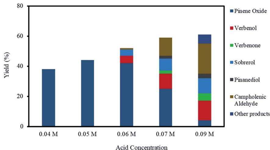
Fig. 5 Effect of acid concentration on  $\alpha$ -pinene epoxidation and distribution of the products. Reaction conditions: temperature (50 °C), reaction time (120 min),  $\alpha$ -pinene (1.25 M),  $\text{H}_2\text{O}_2$  (1.25 M),  $\text{Na}_2\text{WO}_4 \cdot 2\text{H}_2\text{O}$  (0.012 M) and toluene (500 mol%).
