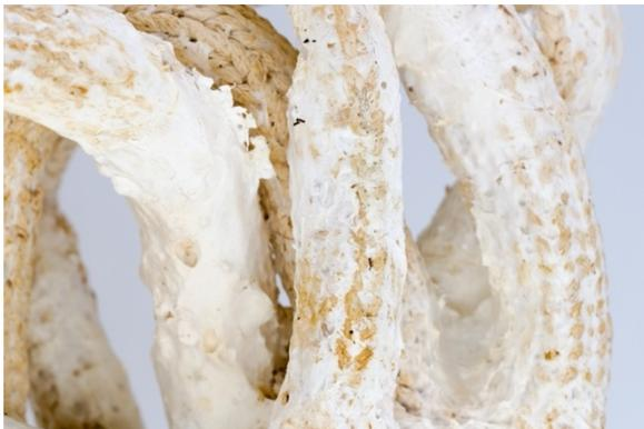
Figure 1: knit mycelium composite using substrate
