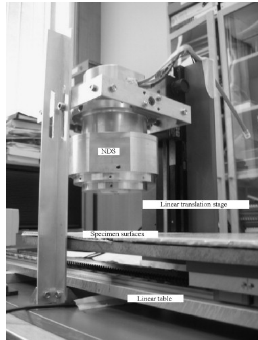
Figure 3: Test platform consisting of the NDS and linear table.
