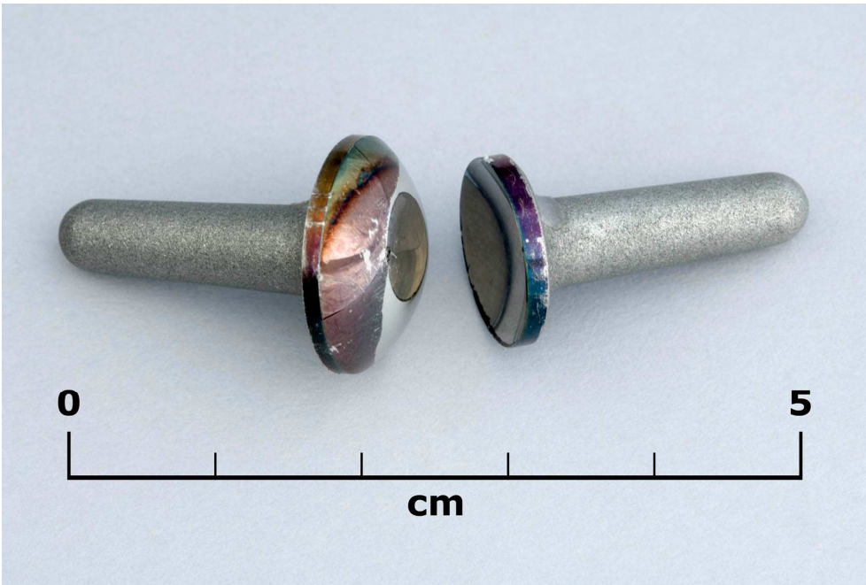
Figure 1 The metal-on-metal MTP prosthesis. The metatarsal component is on the left, the phalangeal component on the right. The remaining DLC coating can be seen on the articulating face of the metatarsal component
