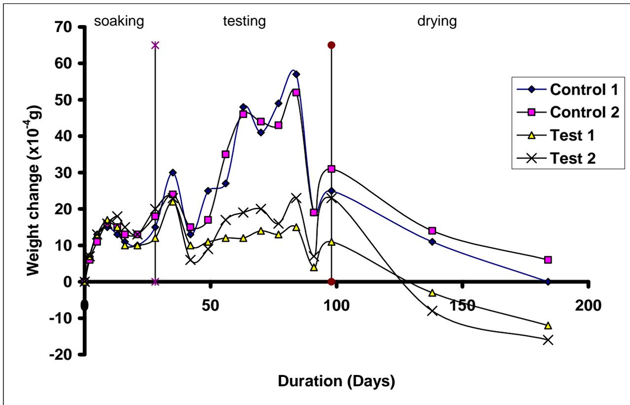
Figure 6 Weight changes over test duration, soaked PEEK metacarpal components.
