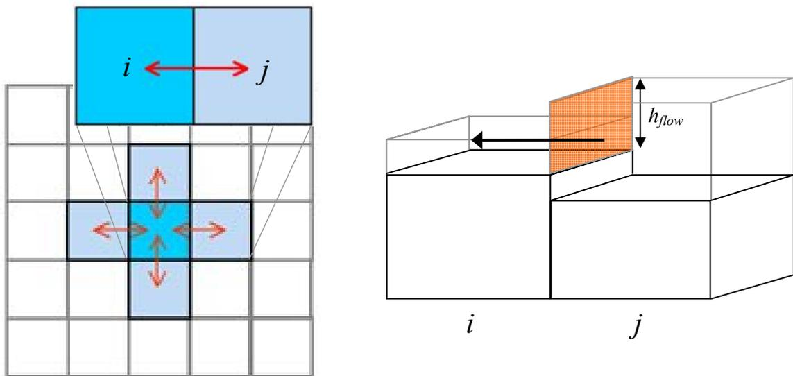
Figure 1: Representation of flow between cells in LISFLOOD-FP.
