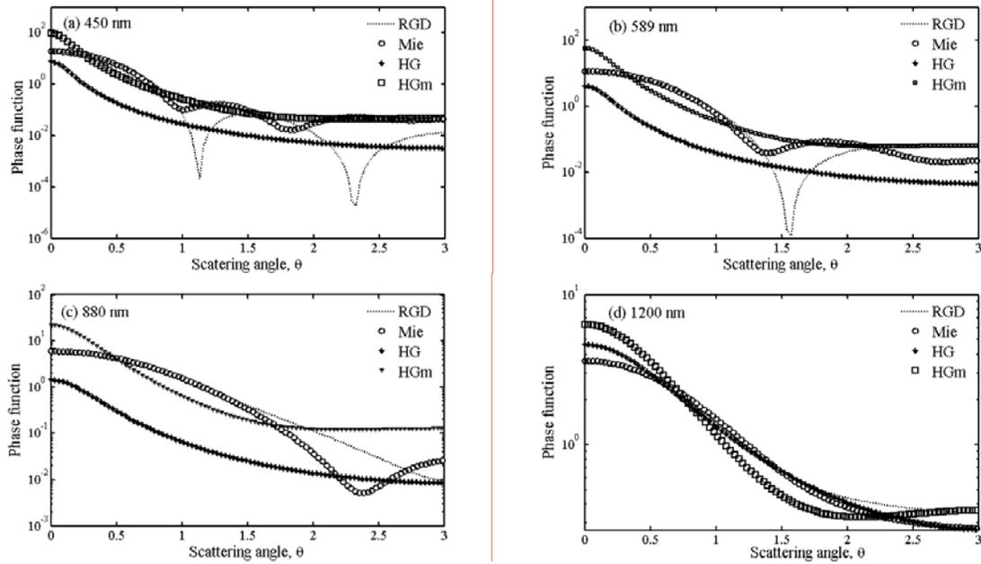
**Figure 7.** Comparison between phase functions computed using Mie, RGD, HG, HGm, for particles of radius,  $a = 0.225 \mu\text{m}$ . (a)  $x = 4.1432$ ,  $g = 0.86$  and  $\lambda = 450 \text{ nm}$ . (b)  $x = 3.1731$ ,  $g = 0.8$  and  $\lambda = 589 \text{ nm}$ . (c)  $x = 2.1238$ ,  $g = 0.69$ , and  $\lambda = 880 \text{ nm}$ . (d)  $x = 1.5574$ ,  $g = 0.44$ , and  $\lambda = 1200 \text{ nm}$ .
