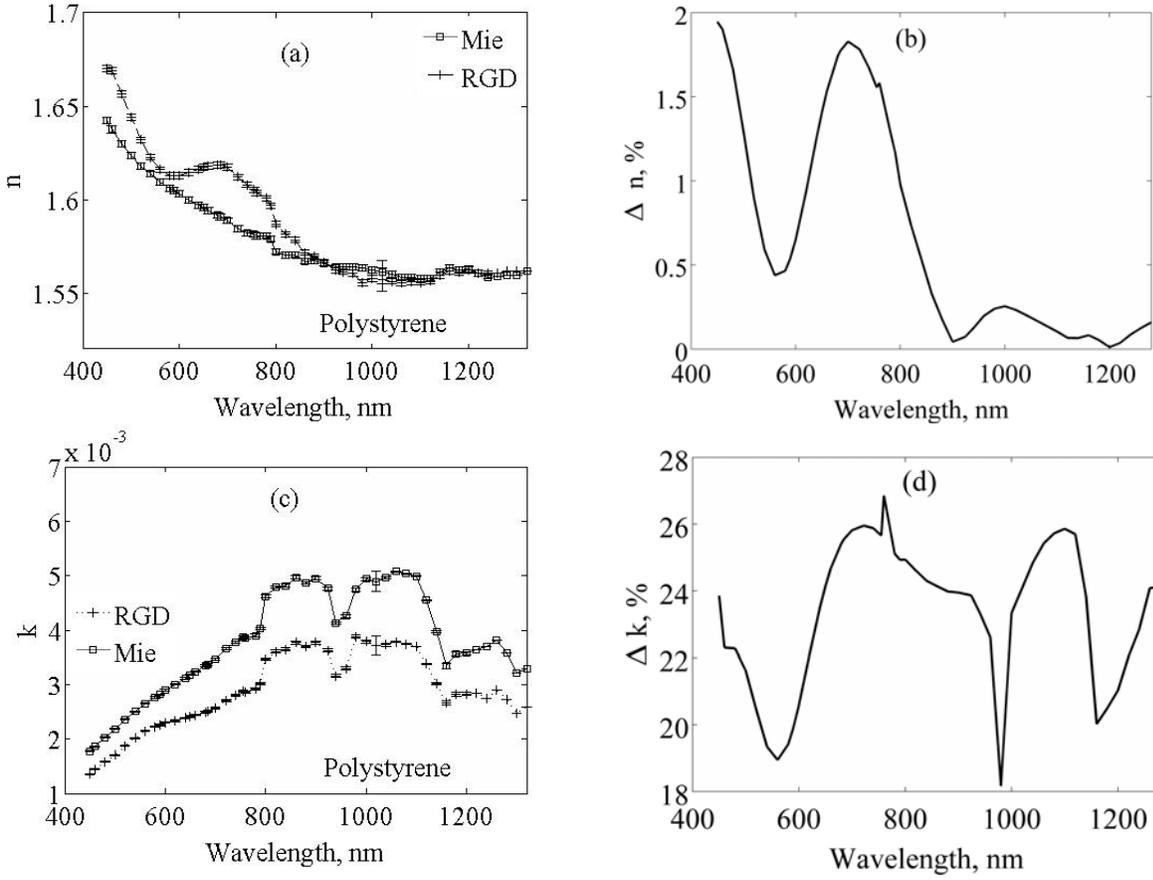
**Figure 2.** Comparison between the complex refractive index estimated using the RGD approximation and the Mie theory for polystyrene. (a) Real part,  $n$ , (b) Percent relative error,  $\Delta n = |n_{\text{mie}} - n_{\text{RGD}}| / n_{\text{mie}} * 100$ , (c) Imaginary part,  $k$ . (d) Percent relative error,  $\Delta k = |k_{\text{mie}} - k_{\text{RGD}}| / k_{\text{mie}} * 100$ .
