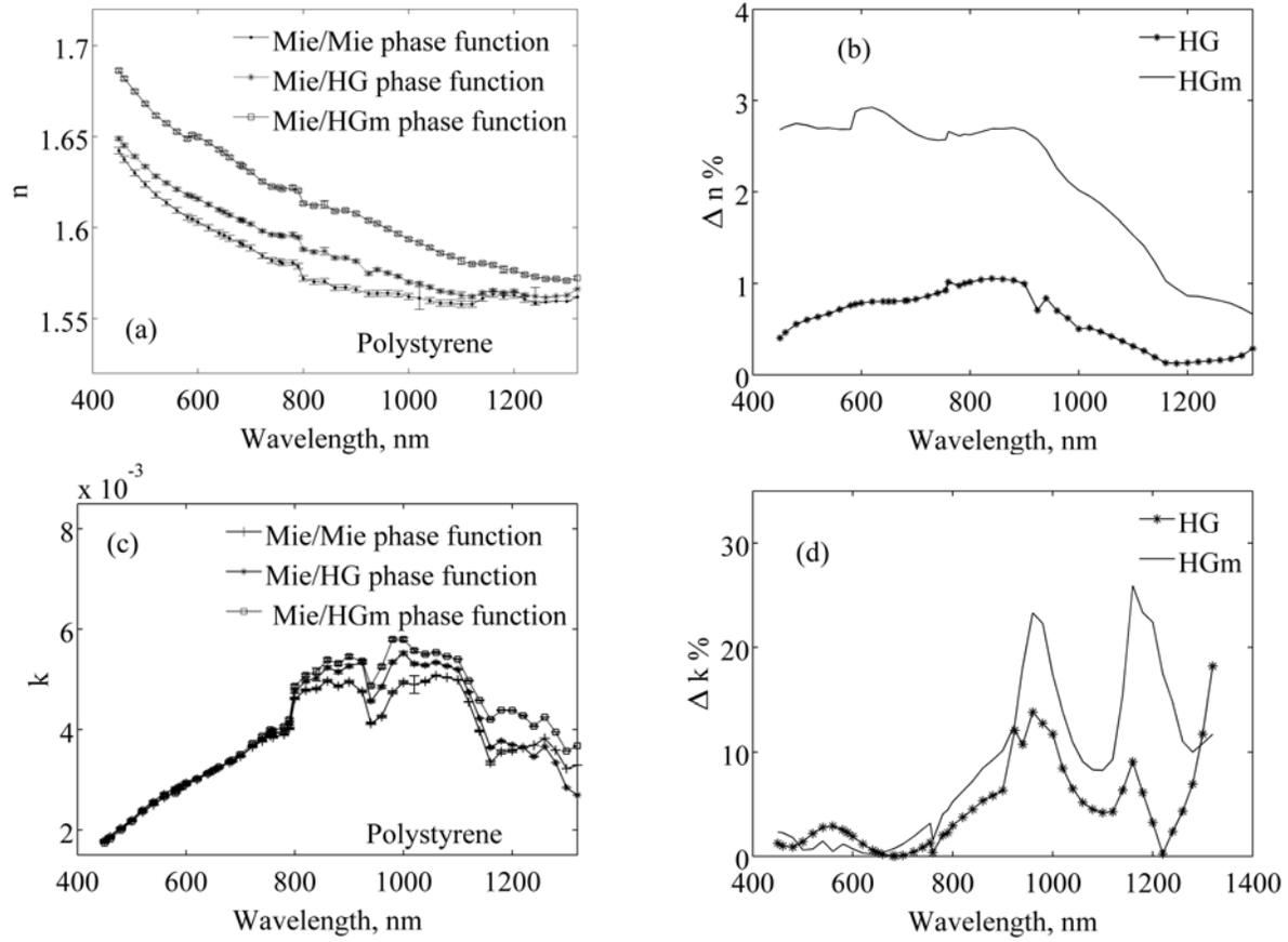
**Figure 4.** Comparison between the optical constants estimated using the Mie phase function, the H-G and the H-Gm approximation for polystyrene. (a)  $n(\lambda)$ . (b) Percent relative error  $\Delta n = \left| n_{\text{mie}} - n_{\text{HG(or HGm)}} \right| / n_{\text{mie}} * 100$ . (c)  $k(\lambda)$ . (d) Percent relative error,  $\Delta k = \left| k_{\text{mie}} - k_{\text{HG(or HGm)}} \right| / k_{\text{mie}} * 100$ .
