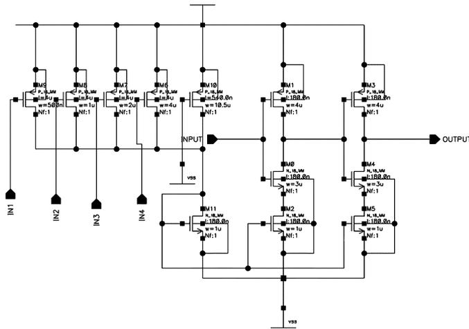
Fig. 3. Variable delay line.
