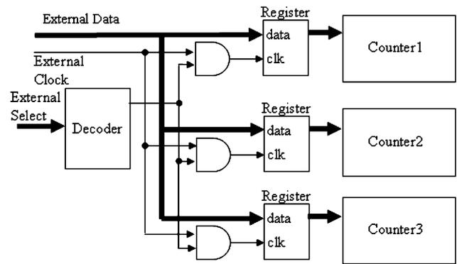
Fig. 7. Loading circuit for controlling counters.
