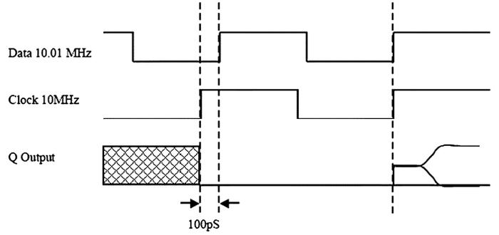
Fig. 1. Traditional measurement method using two oscillators.
