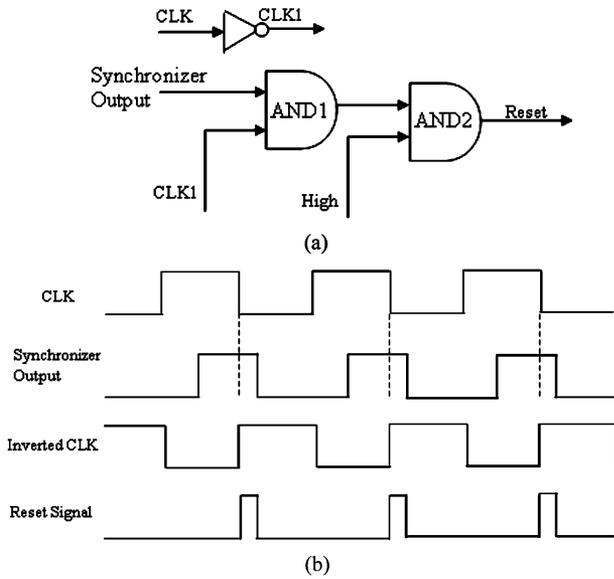
Fig. 8. Generation of RESET signal.
