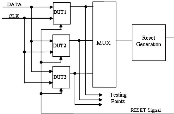
Fig. 5. Multiplexer circuit for DUTs.
