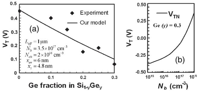
Fig. 7. (a) Comparison of  $V_T$  values extracted from the present model with experimental data for different Ge fractions in a relaxed  $\text{Si}_{1-y}\text{Ge}_y$  VS ( $y$ ) for n-MOSFETs in a single-channel architecture. (b) Variation of  $V_T$  with  $N_b$  for these devices with a Ge content  $y = 0.3$ .
