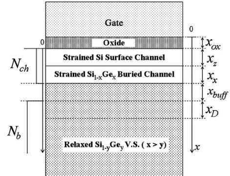
Fig. 1. Schematic cross section of a  $\epsilon$ -Si/ $\epsilon$ -Si<sub>1-x</sub>Ge<sub>x</sub>/relaxed Si<sub>1-y</sub>Ge<sub>y</sub> ( $y < x$ ) dual-channel CMOS architecture.
