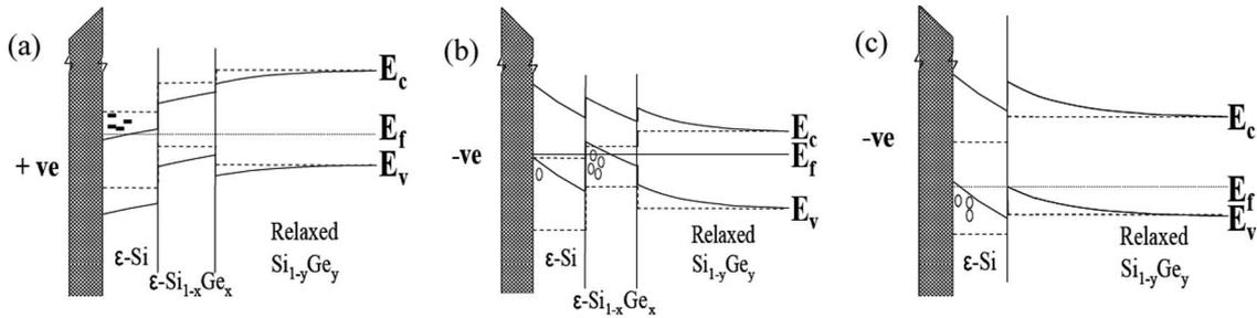
Fig. 2. Schematic band diagram for (a) n-MOSFETs and (b) p-MOSFETs in a dual-channel architecture and (c) p-MOSFETs using a single-channel architecture.
