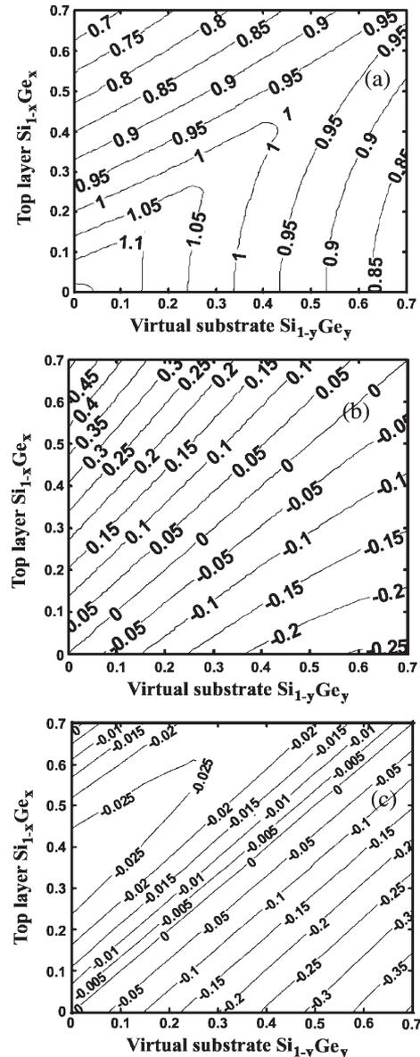
Fig. 3. Contour plots of the calculated generalized band parameters. (a) Band gap. (b) Valence band offsets. (c) Conduction band offsets.
