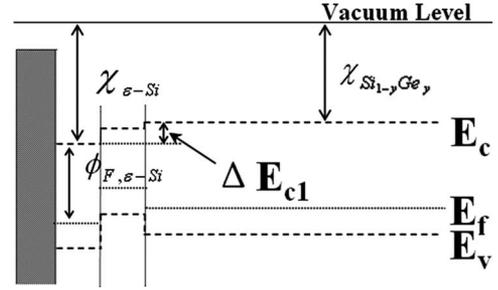
Fig. 4. Schematic band diagram showing the work function of a semiconductor in a dual-channel architecture.
