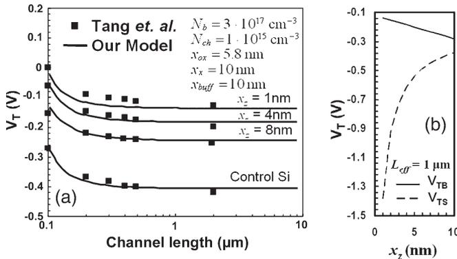
Fig. 8. (a) Comparison of  $V_T$  values calculated from the present model with experimental data [19] at different effective gate lengths  $L_{\text{eff}}$  for p-MOSFETs in  $\text{Si}/\varepsilon\text{-Si}_{0.7}\text{Ge}_{0.3}$  on Si architectures with 1, 4, and 8 nm strained Si layer thicknesses  $x_z$ . (b) Variation of  $V_T$  with  $x_z$  for  $L_{\text{eff}} = 1 \mu\text{m}$ .
