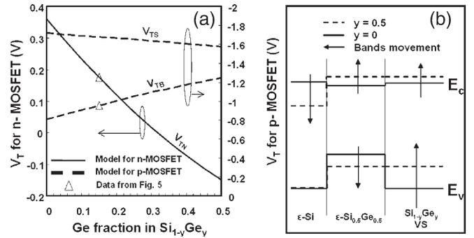
Fig. 9. (a) Plots of  $V_{\text{TN}}$ ,  $V_{\text{TB}}$ , and  $V_{\text{TS}}$ , calculated using the present model for different Ge fractions in the  $\text{Si}_{1-y}\text{Ge}_y$  VS ( $y$ ) for both n- and p-MOSFETs in a  $\varepsilon\text{-Si}/\varepsilon\text{-Si}_{0.5}\text{Ge}_{0.5}$ /relaxed  $\text{Si}_{1-y}\text{Ge}_y$  VS dual-channel architecture. (b) Schematic energy band moment for increasing the Ge fraction ( $y$ ) from 0 to 0.5.
