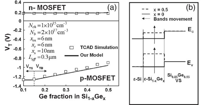
Fig. 5. (a) Comparison of  $V_T$  values extracted from the present model and TCAD simulation at different Ge fractions in a Si $_{1-x}$ Ge $_x$  buried channel for the CMOS devices on a  $\epsilon$ -Si/ $\epsilon$ -Si $_{1-x}$ Ge $_x$ /relaxed Si $_{0.85}$ Ge $_{0.15}$  VS architecture. (b) Schematic energy band moment for increasing Ge fraction ( $x$ ) from 0 to 0.5.
