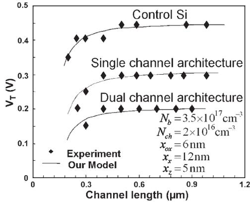
Fig. 6. Comparison of  $V_T$  values extracted from the present model with experimental data at different effective gate lengths for n-MOSFETs on control Si,  $\epsilon$ -Si on a Si<sub>0.85</sub>Ge<sub>0.15</sub> VS in a single-channel architecture, and  $\epsilon$ -Si/ $\epsilon$ -Si<sub>0.7</sub>Ge<sub>0.3</sub> on a relaxed Si<sub>0.85</sub>Ge<sub>0.15</sub> VS in a dual-channel architecture.
